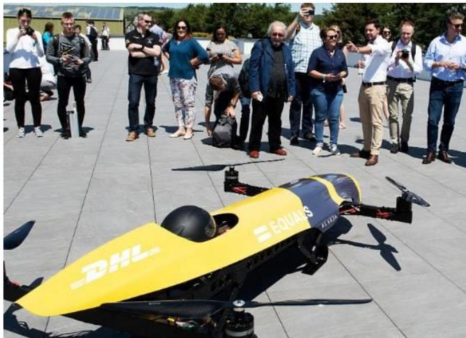
Swappable battery pack lasts 15 minutes at full power. Alauda Racing, the Australian start-up company behind the series, says the finished machines will be able to hit 200kmh. The Speeders are around four metres long, weigh 250kg and are propelled by eight 50kW motors driving 60-inch blades. The 500kWh battery packs provide full thrust for 15 minutes and are "swappable", meaning that they can be refreshed during pit stops for the 30-minute races.
