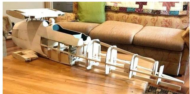
The rudder and Elevator servos are above the bottom wing with the idling arms and adjustment clevises accessed through a nice big hatch just behind the wing. All the control services, (even the left and right Elevators are separate) are closed loop using the Du-Bro Heavy Duty Dual Pull -Pull System. I've fitted all six guide tubes so I just have to slide the wires through after covering etc.
